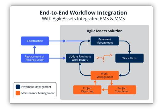
After pavement construction is complete, the pavement enters the pavement management cycle. Over time, the pavement will need maintenance work. The pavement management team analyzes the pavement network and creates work plans, which the maintenance team uses to generate work orders. The maintenance crew completes the work orders and updates the work data on the maintenance side. With the integrated solution, the work status also gets updated in the pavement management system.
